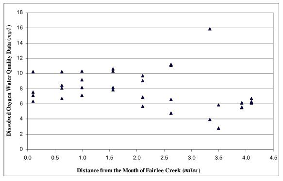
Figure 6: Longitudinal Profile of Dissolved Oxygen Data
