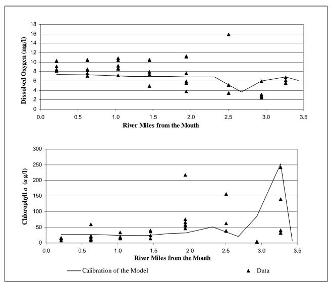
Figure 10: Results of the Calibration of the Model for Chlorophyll a and Dissolved Oxygen
