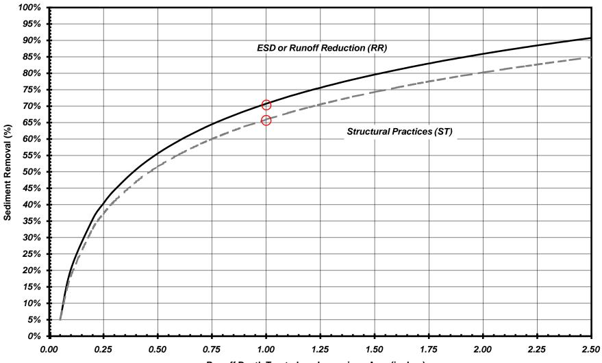
Sediment Removal for ESD (RR) and Structural (ST) Stormwater Practices
