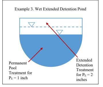
WM credit is available for extended detention volume above the permanent pool volume for up to a total rainfall depth treated of 3 inches:
