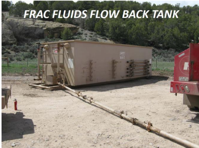
Figure 7: Flowback Tanks (Photo courtesy of the Colorado Oil and Gas Conservation Commission)
