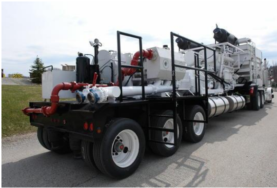
Figure 6: Hydraulic Fracturing Pumps (Photo courtesy of http://www.jibodies.com )
