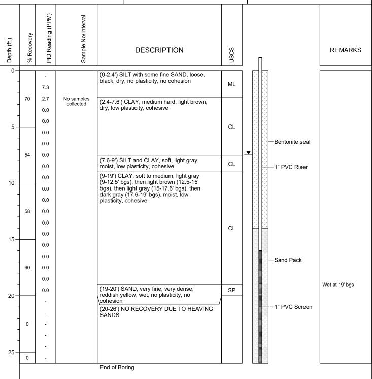
Boring terminated at 26' bgs due to groundwater and piezometer installation
