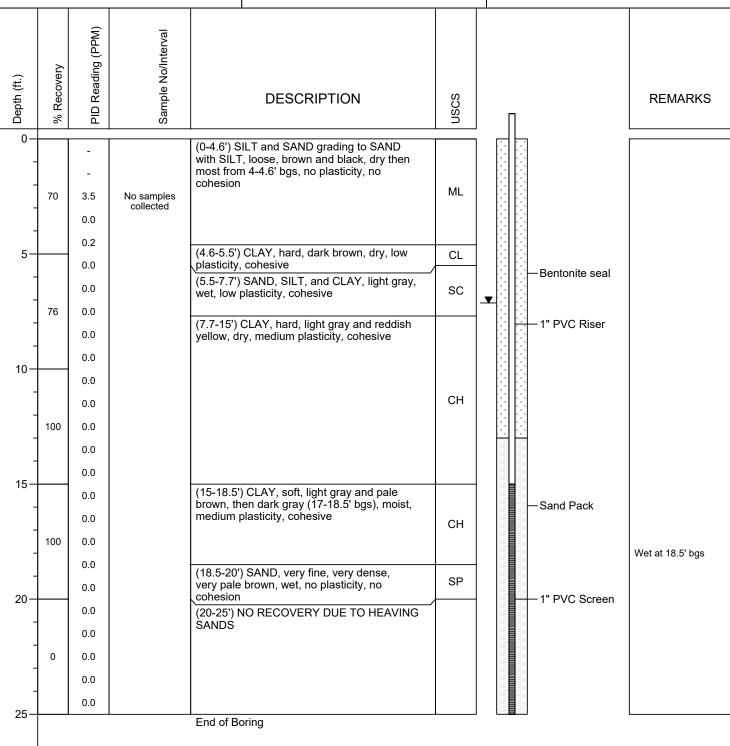
Boring terminated at 25' bgs due to groundwater and piezometer installation
