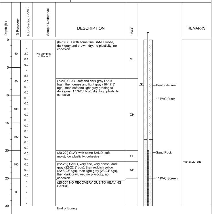
Boring terminated at 30' bgs due to groundwater and piezometer installation
