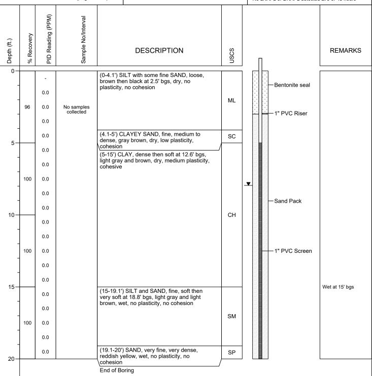
Boring terminated at 20' bgs due to Work Plan
