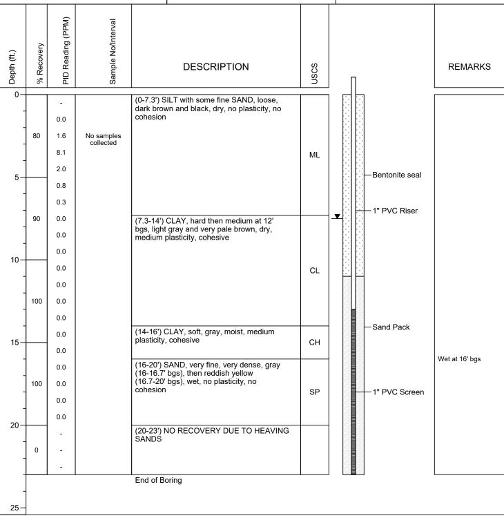
Boring terminated at 23' bgs due to groundwater and piezometer installation
