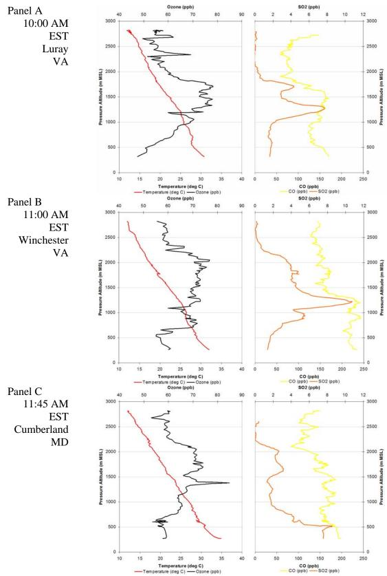
Figure 11.2.6 Aircraft spirals on August 15, 2005. Ozone is in black, temperature is in red, SO2 is in orange, and CO is in yellow.
