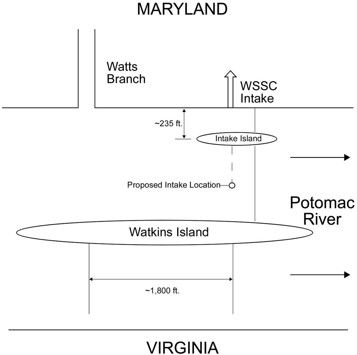
Figure 1: A schematic view of the area near the WSSC intake. This figure is not to scale, y-axis has been exaggerated to provide adequate detail at the intake.
