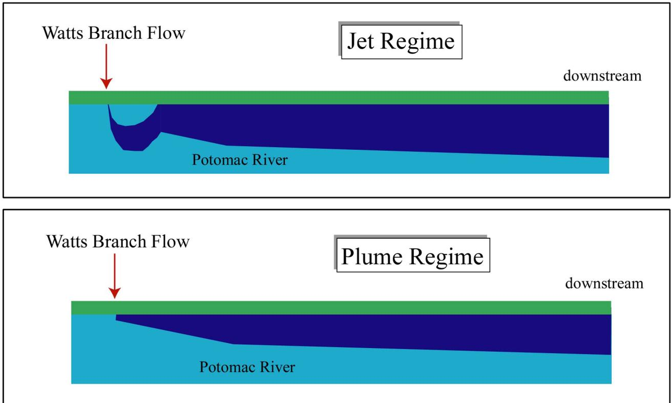
**Figure 13 – Mixing Zone Model of Watts Branch Flow**
