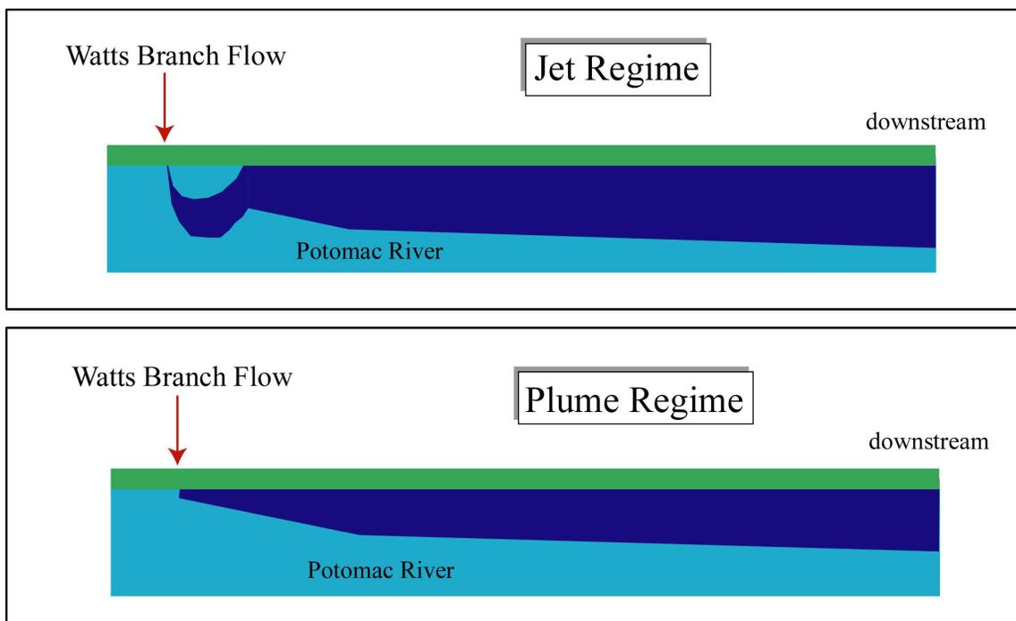
Figure 3: A schematic example of the jet and plume regimes produced by CORMIX
