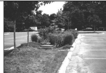
Figure 10 - Parking Lot Island Turned into Bioretention
