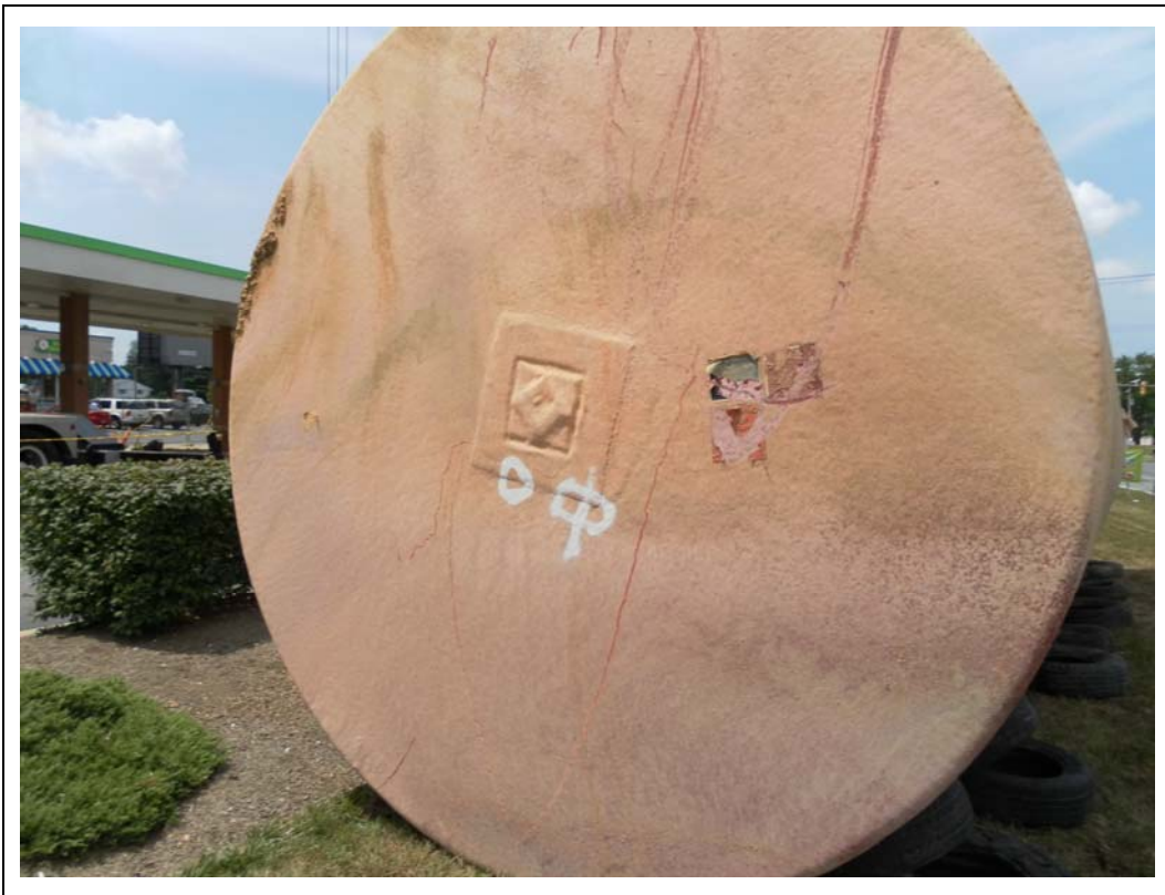
Photograph 10: View of north end of 20,000-gallon UST, with three suspect pinholes in FRP circled with white paint.
