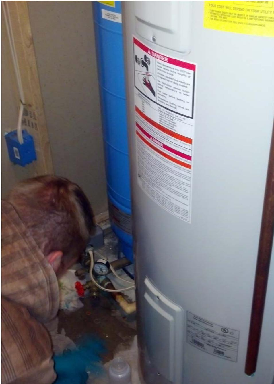
Sample collection from pressure tank drain.
