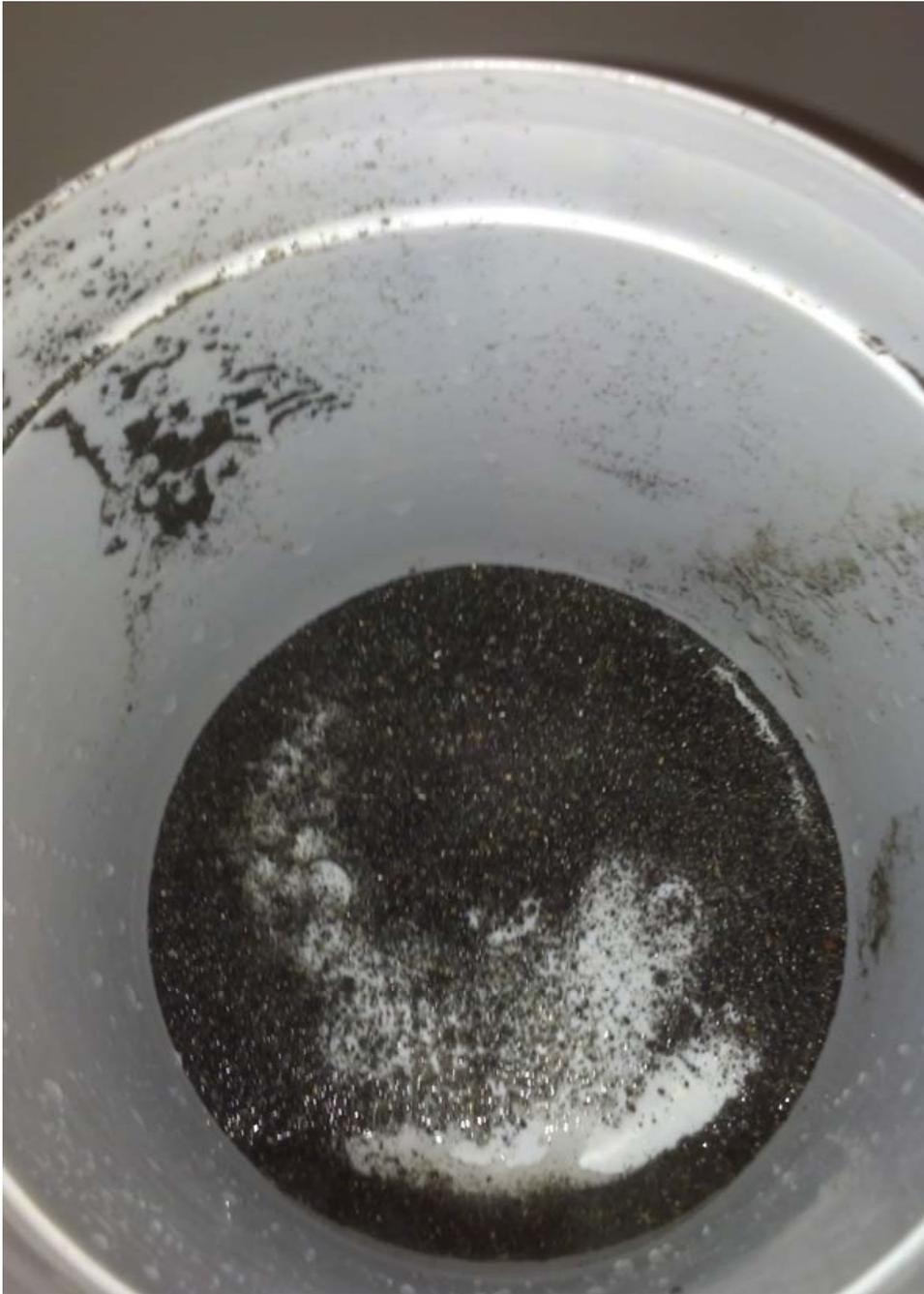
Sediment from pressure tank drain cycles #2 and #3
