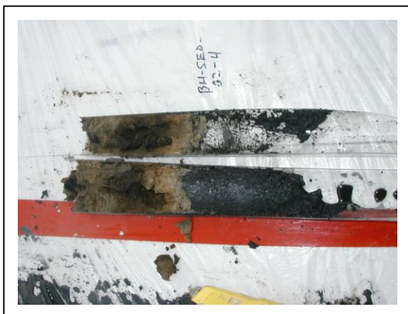
Figure 6. Fill material (right) on top of tan/dark tan sand (left)
