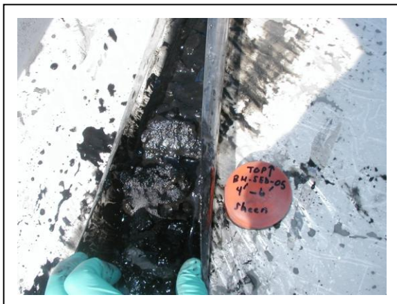
Figure 10. Sheen present in core, negative Sudan IV test for NAPL
