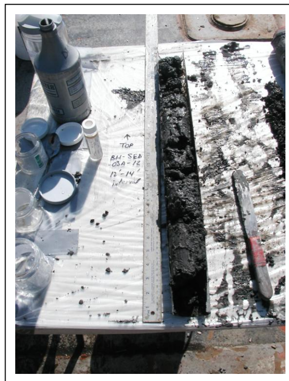
Figure 7. Fill material from offshore location 3A, 12-14 feet below the sediment surface
