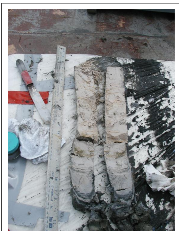
Figure 8. Twenty-two (22) feet below the sediment surface. Fine sands and hydrocarbon odor.
