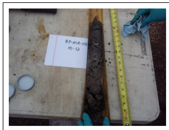
Figure 6. Soil core which tested positive for NAPL with Sudan IV test.
